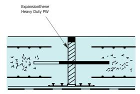
Water retaining structure wall expansion joint
