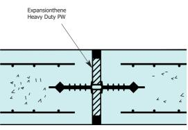
Water retaining structure floor expansion joint
